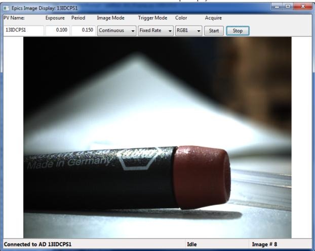
The fields and buttons on the top control several Area Detector settings, such as starting and stopping the acquisition.
