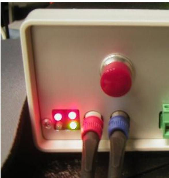
After step (4) above, the VME receiving continuous data via the orange fiber, to the bottom channel 0 of the FIBER2. The ADCMOD's top left light indicates data is flowing from it.
