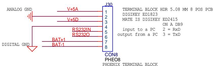
Pin 1 is on the right in the photo. At present pins 5-8 are not used - they will eventually control the battery supply.
