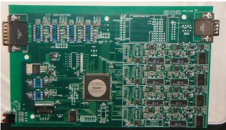
FIG 2C. A photograph of the current amplifier method for electrometers. This board holds four chains of electrometer current amplifiers. Data is digitized, and can be packaged in a way consistent with the charge amplifiers. There are V/F converters on this board but this is not a desired development path, ADC's and digital signal averaging are better.
