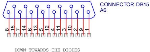
DB15 CONNECTOR, PLACED ON THIS SIDE OF PCB
