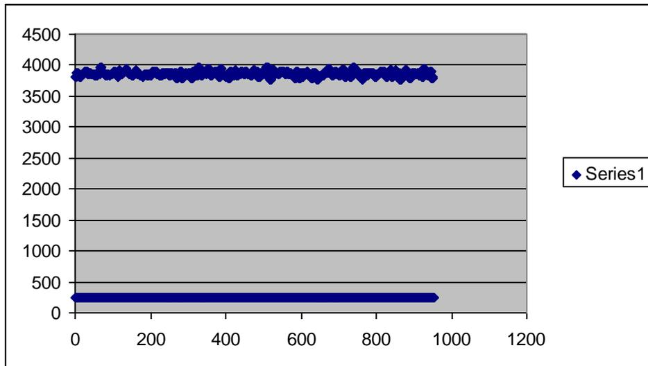
Jim Ciston and Mark Rivers at sector 13 applied the BPM to measure the vibrations, and mechanical stability of their beam. They used 800Hz data. This electrometer system is very low noise at quite good bandwidth. Mark has an EPICS PID control loop system for feedback stabilization of the beam. [Ref: Performance Analysis of a Backscattering Fluorescence BPM on 13ID, James Ciston 12/22/2003, internal report to Mark etc.]
