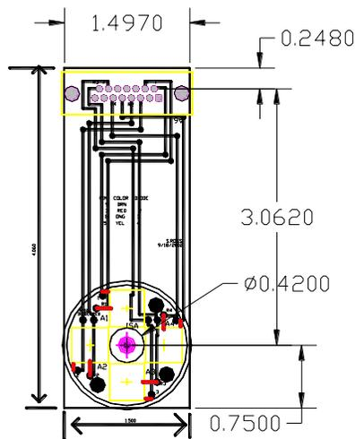
FIG 1 B,C A photograph, and a drawing of the diode6 design. This printed circuit board fits into a KF50 cross and positions the diodes in the center. Standoffs hold a second circuit board approximately 1 cm. above it and this circuit board holds the foil. This is a very simple one-piece design for medium vacuum conditions. Pinout given in section 7.
