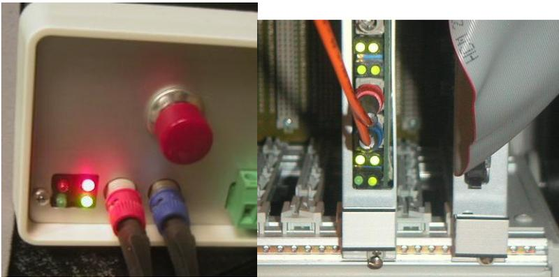
ADCMOD upon power up, but before it starts to transmit data. After the six steps above, 3 FIBER2 lights would be on: the bottom right, now flickering, would be solid. In this photo FIBER2 has only top 2 lights glowing because ADCMOD has not yet been turned on.
