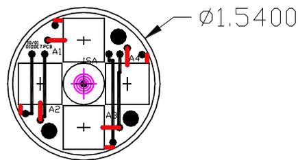
FIG 1A This is the basic printed circuit board type design (DIODE5) holding the four UDT 1 cm<sup>2</sup> PIN diodes. It is about as small as possible with these diodes. The center hole is milled out to about 0.5 inch diameter. This circuit board fits into a KF-40 or KF-50 size vacuum system.
