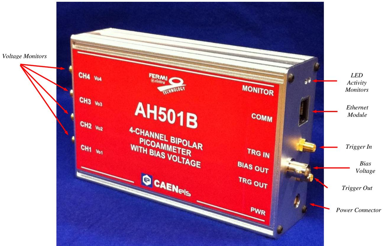
Fig. 1 - The AH501C I/O Connections
