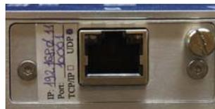
Fig. 3 - "ETHERPiggy" Module with label
