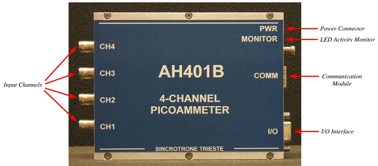
Fig. 1 - The AH401B I/O Connections
