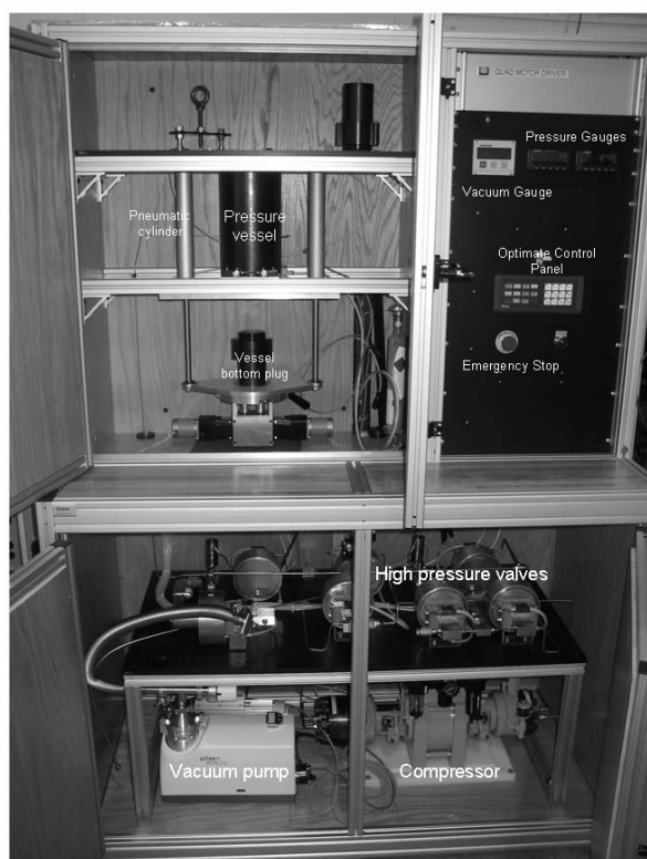
Fig. 2. Annotated photograph of gas loading system
