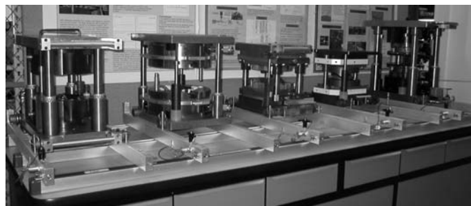
Fig. 1. Various large-volume high pressure devices for experiments in the 250 T press in 13-BM-D.
