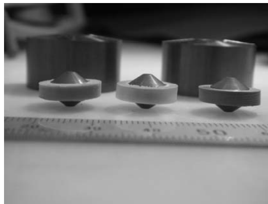
Fig. 2. High pressure cell with three kinds of plastic ring gaskets.
