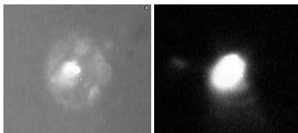
Fig. 3. Optical micrographs of the sample region in a hybrid DAC during heating (left: with light, right: without light).
